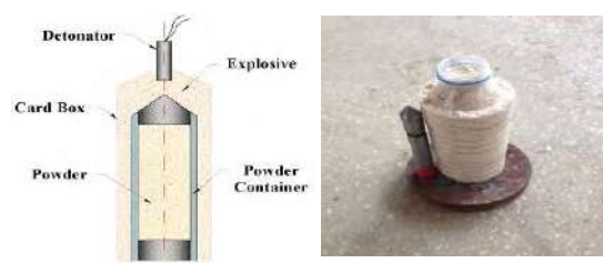
Fig.2 Axis-Symmetric Cylindrical Set-up for explosion consolidation of HEAP.
