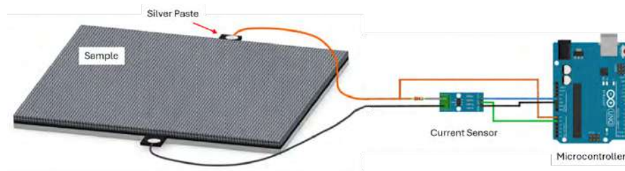
Figure 1. Schematic illustration of the damage monitoring configuration for CARALL composites
