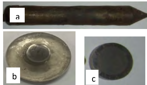
Fig. 3. View of Bulk composite samples obtained by explosive consolidation of FeWAlTiNi: a) steel container after explosion loading; b) Bulk sample by mechanical treatment for removal of steel jacket; c) FeWAlTiNi Bulk composite.
