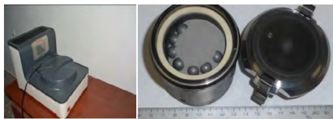
Fig.1. MA of 15%Fe-45%W7%Al-12%Ti-15%Ni-3%C-3%B: a) Ball mill view; b) Blend view Charged in jar.
