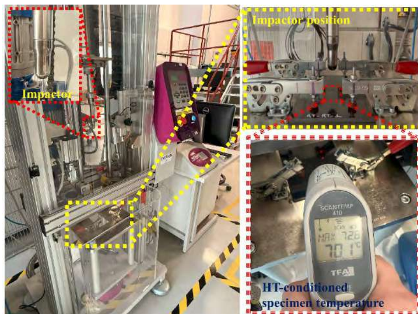
Figure 2. Drop tower test setup with specimen positioning and temperature monitoring for HT-conditioned specimen.
