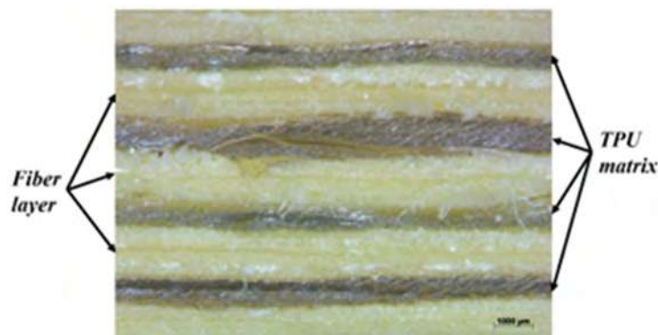
Fig. 1. Optical microscopy image of TPU composite in cross-section.
