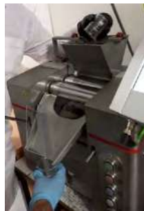
a) three-roll milling process to ensure homogeneous dispersion
