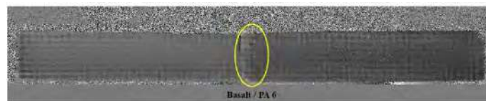
Fig. 2 Shearogram after flexural test of basalt/PA specimen.
