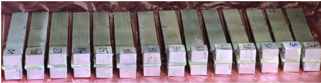
Figure 1: The composite coupons (virgin) for the DCB tests (3, 6 and 9 mm/min).
