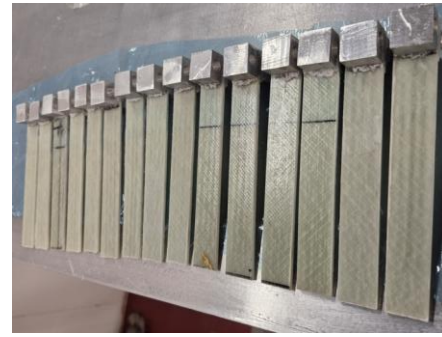
Figure 1: The composite coupons (virgin) for the DCB tests (3, 6 and 9 mm/min).
