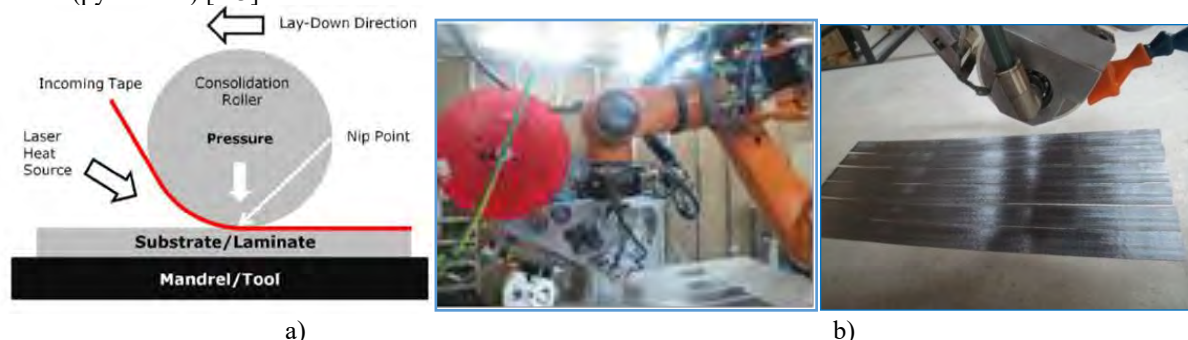
Fig. 1. a) Schematic representation of automatic tape laying process b) Automatic laser-assisted UD laying
