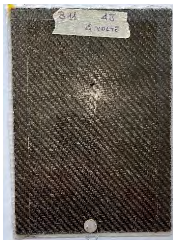
Fig. 1. Photo of impacted sample (4J impact × 4) with surface bonded sensor
