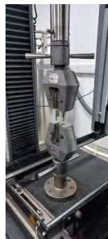
Fig. 1. Tensile testing of specimens on Instron 8872 model tensile machine
