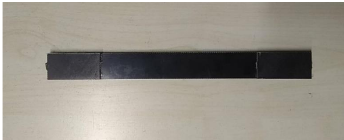
Fig. 2. Basalt fiber-reinforced specimen (after tabbing)
