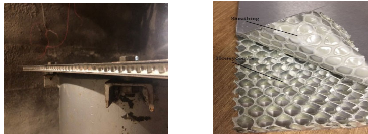
Figure 1. Steel plate with an aluminum honeycomb layer
